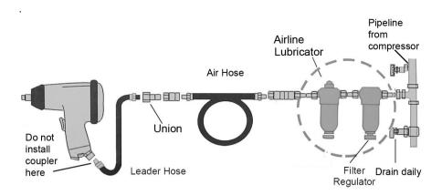
A typical air line layout is shown above. If an automatic in-line filter/regulator is used it will keep the tool in good condition. The lubricator should be adjusted to approx 2 drops per minute and SAE 10 oil should be used.
